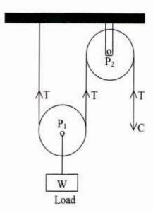
The above figure shows the combination of a movable pulley  $P_1$  with a fixed pulley  $P_2$  used for lifting up a load W.
